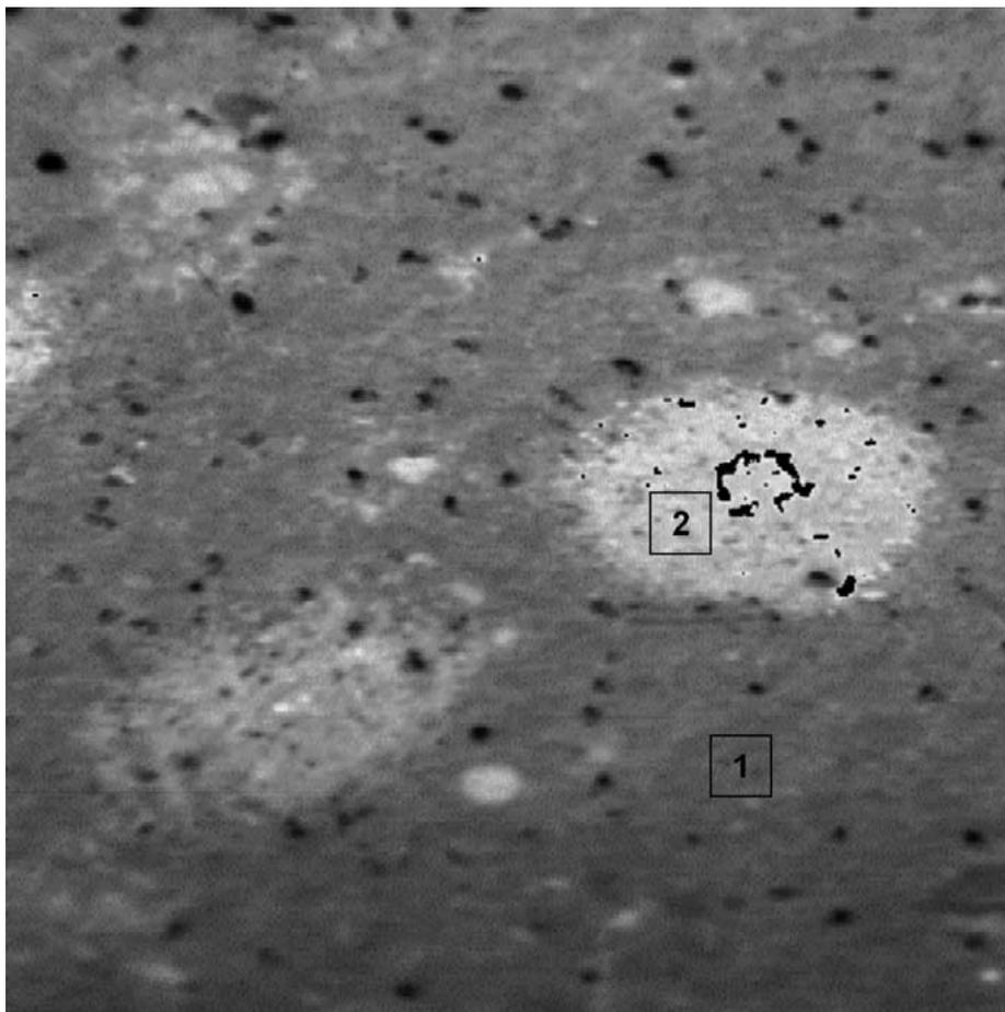
Figure 3 Scanned Auger Oxygen Map;  $400 \times 400 \mu\text{m}$  region from dulled gold surface including dark spots. Surface oxide concentrations are highest in regions corresponding to the dark spots.
