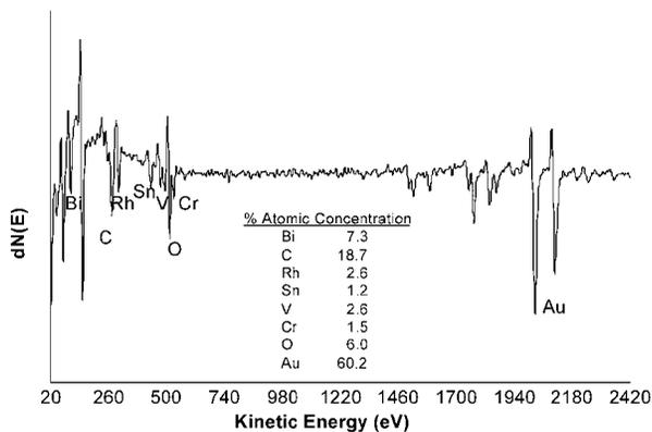
Figure 4 Auger wide survey spectrum of Inconel 625 with Au thin film as received, no thermal exposure; Analysis taken from surface area with bright gold appearance.
