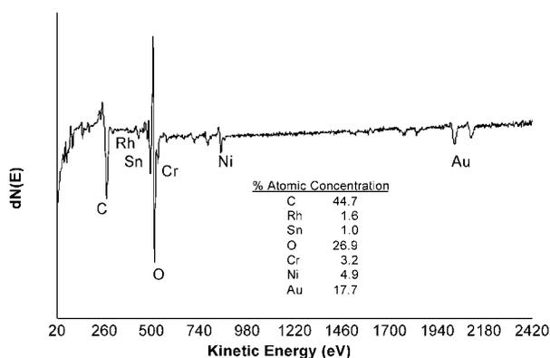
Figure 6 Auger wide survey spectrum of Inconel 625 with Au thin film; Analysis taken from dark spots appearing through the dull gold region after 924 hours of heat exposure at 590°C.
