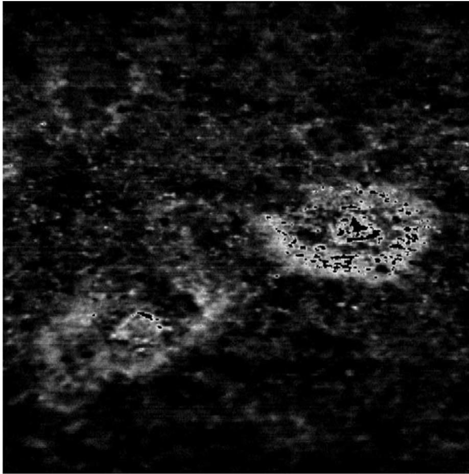
Figure 2 Scanned Auger Nickel Map;  $400 \times 400 \mu\text{m}$  region from dulled gold surface including dark spots. Ni concentrated in light regions.
