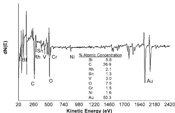
Figure 5 Auger wide survey spectrum of Inconel 625 with Au thin film; Analysis taken from surface area appearing as dull gold after 924 hours of heat exposure at 590°C.
