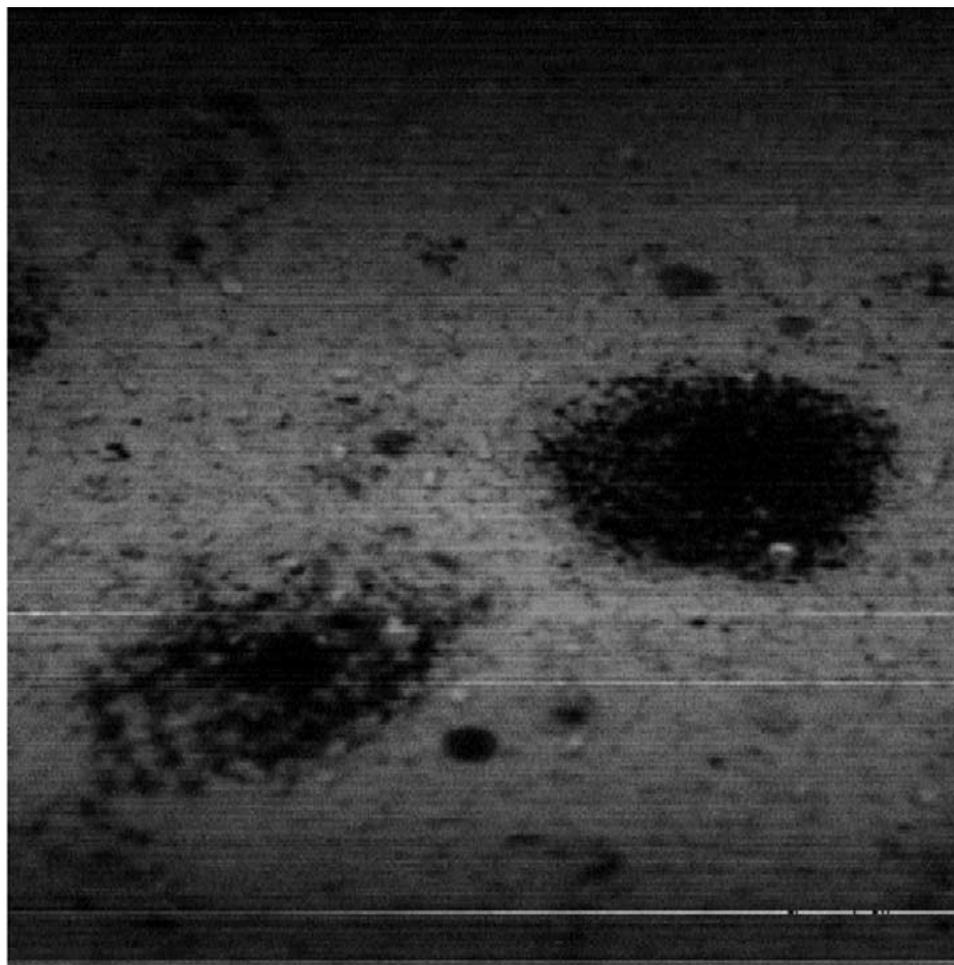
Figure 1 Scanned Auger gold map;  $400 \times 400 \mu\text{m}$  region from dulled gold surface including dark spots. Light areas correspond to Au.
