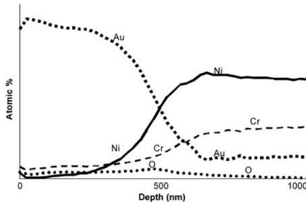
Figure 7 Auger depth profile of the dull gold region after 924 hours of exposure at 590°C.
